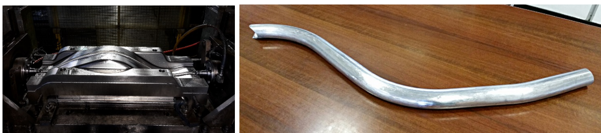
Fig. 3: Hydroforming die fitted to the Schuler press (left), hydroformed tube (right)
