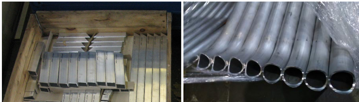
Fig 2: Trimmed elements of rectangular shaped tubes (left), bended and machined circular shaped tubes (right)
